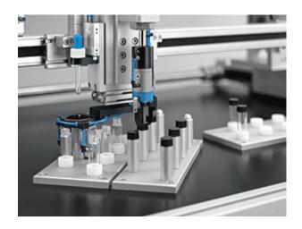
Festo presented a number of systems designed to automate clinical laboratory processes. The new capper/decapper two-station system reduces ergonomic stress for laboratory technicians. The technician can set the sample in the holder and then push the drawer to the closed position to begin the cycle. Highlights of this system include choice of tube sizes, three functions (rotary, linear, gripping) in one, safety interlocks, and the ability to customize the automation surrounding the unit.
