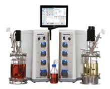
Suitable for microbial and cell culture, scale up to scale down, batch, fed-batch, and continuous processes and with left- and right-handed orientation, the BioFlo 320 is designed to meet the needs of the biotech and pharmaceutical industries.
