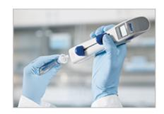
The Repeater M4 dispenses 1  $\mu$ L to 10 mL, and since there are 20 volume settings for each of the nine Combitips, there are a maximum of 100 dispensing actions, making it applicable for 96-well plates.
