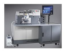
The Intellisort II sorter eliminates the need for bead-based drop-delay routines, which alleviate the need to remove sterile samples during drop-delay recalculation due to nozzle blockages. Intellisort II's ability to maintain droplet breakoff for uninterrupted aseptic sorting helps preserve sort integrity.
