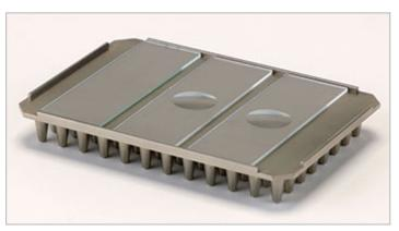
The adapter is a single piece of precision-engineered aluminum that is designed for the easy removal of glass slides via the corner cutouts. The aluminum perimeter ridge makes it compatible with the thermal cycler lid, reducing the risk of damage to glass slides and PCR samples if the lid is closed.
