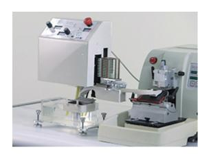
**December 2014—Aquaro Biosystems introduced its PaceSetter section** mounting system, a benchtop instrument that automates the transfer of paraffin-embedded tissue sections directly from microtomes to glass slides.
